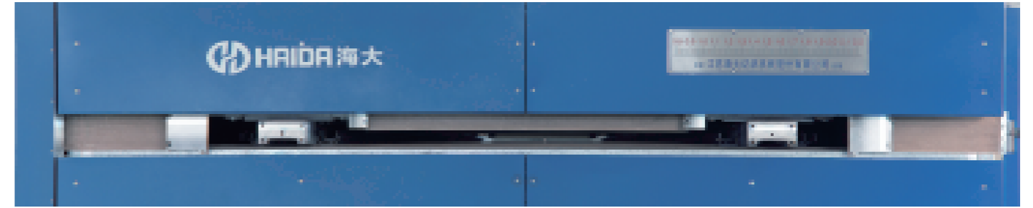
烘箱进口气流屏蔽装置 Cold air barriers in the fabric inlet and outlet
