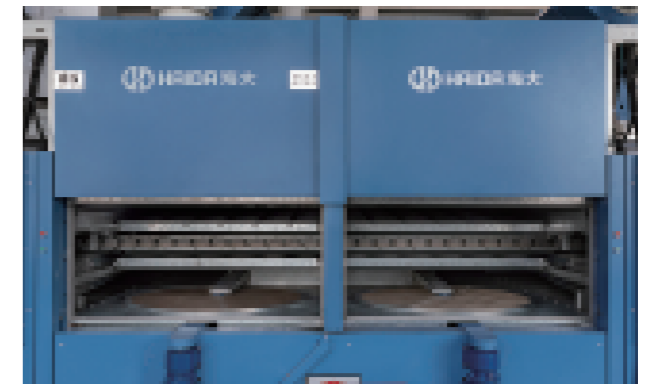
气动升降门, 减少对安装空间的需求, 提升热效率 Pneumatic lifting door, reduces space requirement increases the thermal efficiency
